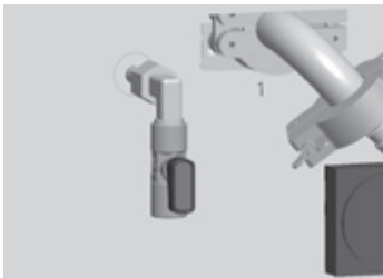
Manual/emergency aeration valve
