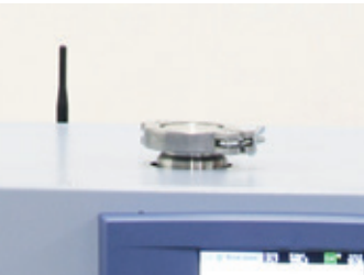
Universal stainless steel access port DIN Ø 40 mm
